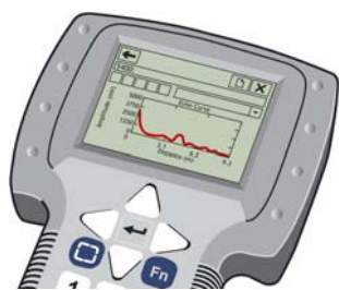
Figure 5 Handheld communicators can also show EDDL graphics
