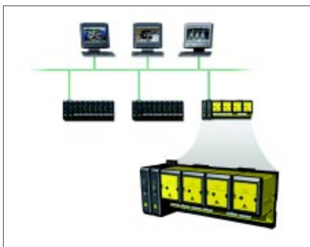
Figure 2 Smart safety logic solver communicates HART
