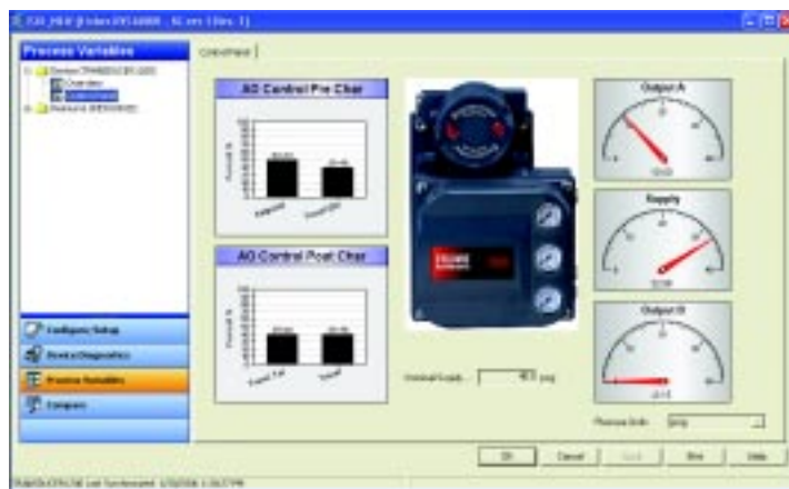
Figure 3 Device management software based on EDDL gives access to information to enable maintenance savings
