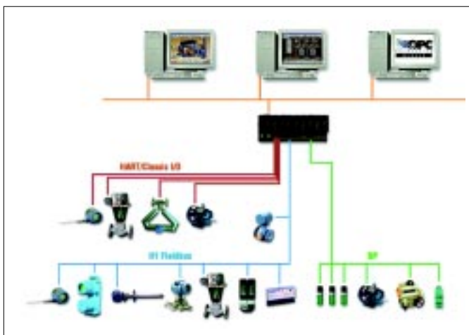
Figure 4 Digital automation system architecture
