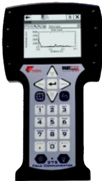
Figure 1 handheld communicator based on EDDL enables field work
