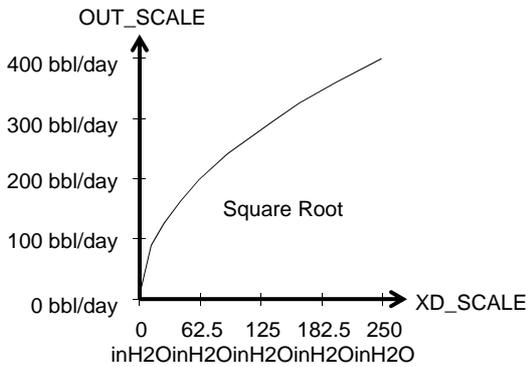
If the pressure transmitter is measuring pressure or DP (L\_TYPE is 'direct'), there is no need to set X\_D\_SCALE. Setting X\_D\_SCALE is only required for DP flow and DP level applications where the transmitter shall convert and scale a DP into flow or level. When L\_TYPE is 'direct' the pressure reading will be seen in the transducer block and on the AI block PV and OUT
