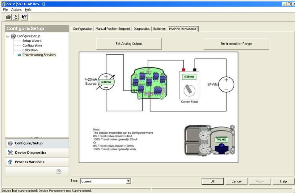
**Figure 8 Positioner manufacturer uses EDDL to illustrate connection for current trim procedure**
