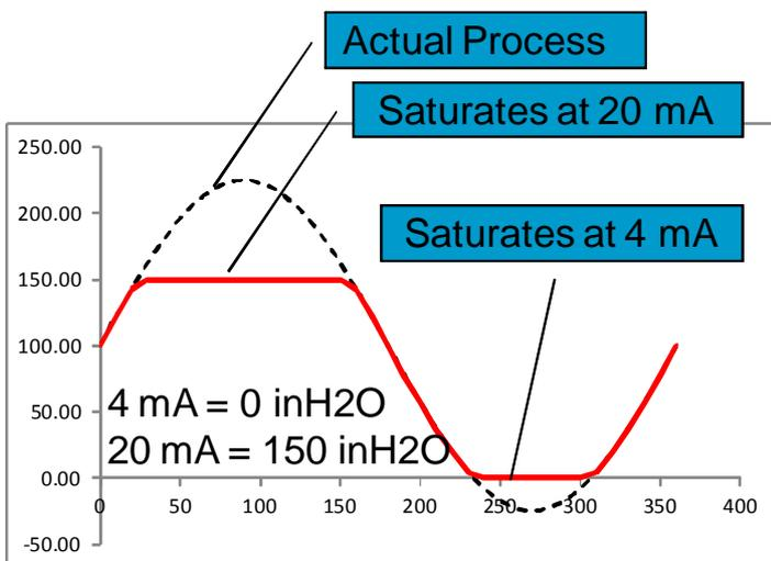
**Figure 2 In an analog signal system the measurement is confined within range values**
