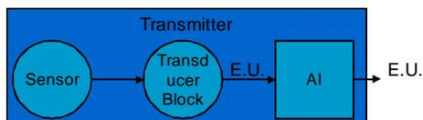
**Figure 5 Digital transmitters internally operate in engineering units**
