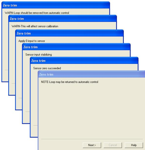
**Figure 11 Calibration wizard is created by the device manufacturer's expert to guide the user**
