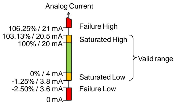
By using transmitters and systems that both conform to the NE43 recommendation, it is possible to flag faults to the operators and control strategies. However, note that all device errors, severe and trivial, are flagged the same way so the operator cannot tell the difference and that if any error occurs it is flagged and the measurement value is not provided.
