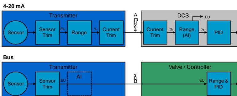
**Figure 4 An analog signal system requires range, current trims, and scaling. A digital bus system does not**
