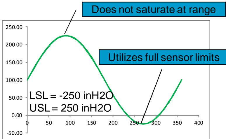
**Figure 3 In a digital bus signal system the measurement enjoys the full sensor limits**
