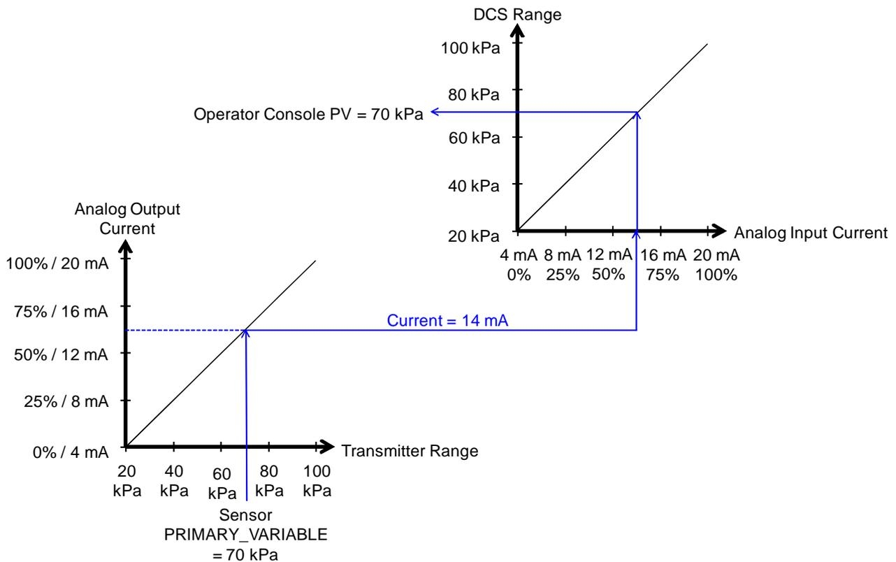
**Figure 1 Range/scaling of transmitter and indication**
