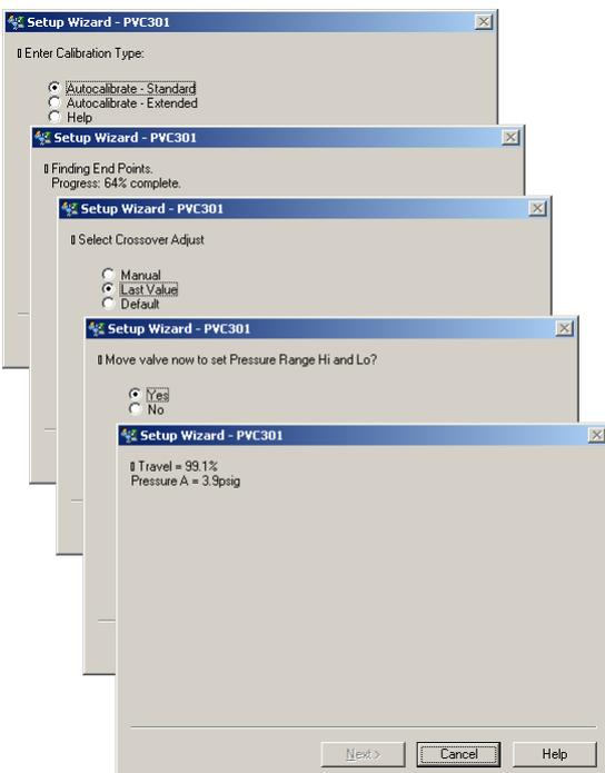
**Figure 9 Automatic valve positioner travel calibration wizard rendered by the system from EDDL**
