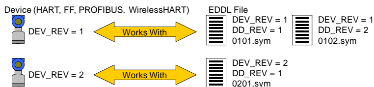
Figure 4 The device manufacturer may improve the user interface without changing the device
